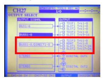
To record in Pro Tools from the DM-24, you must assign your Pro Tools tracks to receive their input from the ADAT connection sent from the DM-24 direct outputs.
